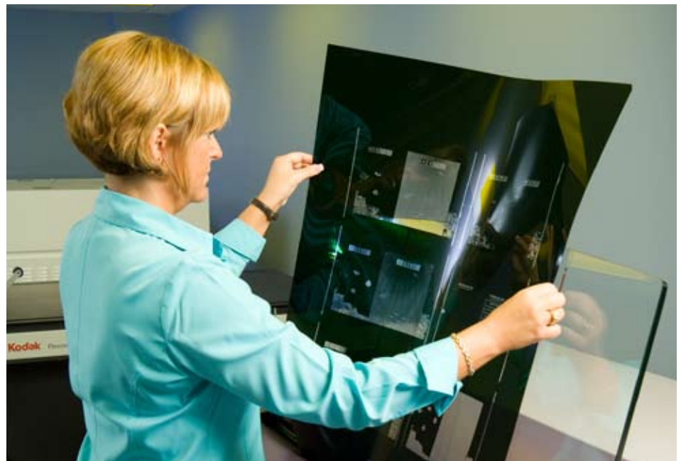
Michelle Gusler pulls an imaged Kodak Flexcel NX Thermal Imaging Layer from LTI's Kodak Trendsetter NX Imager , which provides high-resolution and fast imaging. Lamination ensures intimate optical contact between the imaged layer and Flexcel NX Plates , enabling 1:1 dot reproduction.
